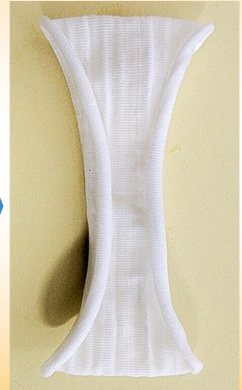
Knitted fabric from CO 2 based TPU yarn
