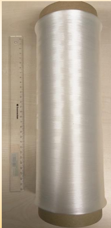
Bobbin with CO 2 based TPU yarn
